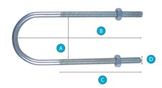
The dimension given for U–bolts is the nominal bore (N.B.) of the pipe. The actual distance between the legs is greater than this to allow for the wall thickness of the pipe. Extended leg U–bolts have approximately 50mm extra thread length on the legs than standard U–bolts. All our U–bolts are supplied with two hex nuts to suit.
