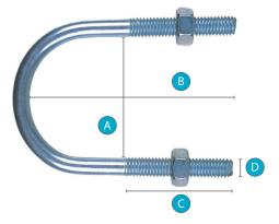
The dimension given for U-bolts is the nominal bore (N.B.) of the pipe. The actual distance between the legs is greater than this to allow for the wall thickness of the pipe. All our U-bolts are supplied with two hex nuts to suit.
